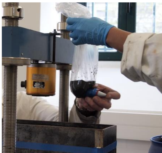
Figure 4 - Paste deposition in the model through a piping device
